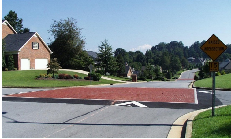
FIGURE 1: RAISED INTERSECTION (SOURCE: GREATER CITY OF PROVIDENCE)
